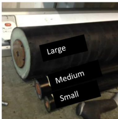
Fig. 2 Photo of the three cables examined, 185, 630 and 2500 mm 2
