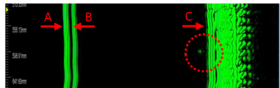
Fig. 5 Contaminant identified in the insulation (not from one of the cables examined in this study)
